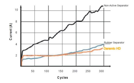
Battery test results with industrial separators 55 °C, IU (2.4 V)
